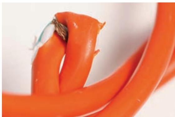
**Crimps or kinks—even in a heavy-duty cord—can cause a break in the protective coating and create a shock hazard.**
