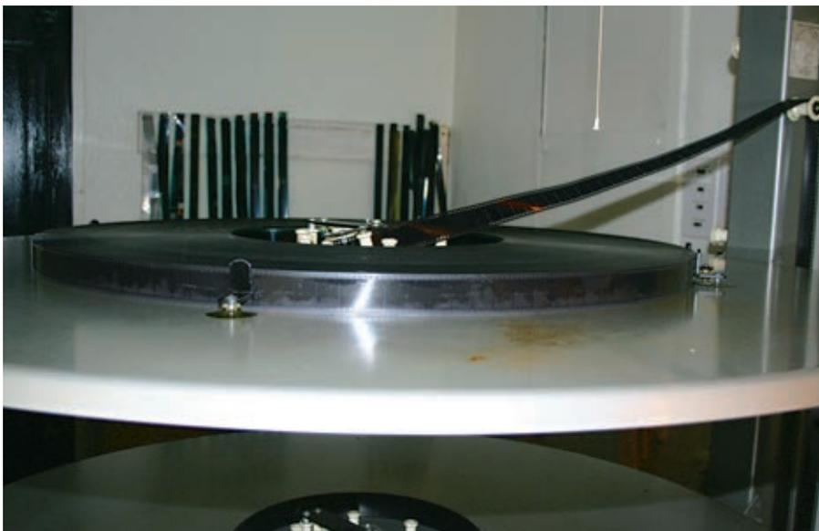
**The film platter machine can accommodate two reels at a time. The six or more reels of each movie are spliced together in the projection room and loaded onto the platters. Once loaded, they have to be previewed in their entirety to be certain that all reels are in the right order and there are no glitches. A new digital format will alleviate the need to load the reels, but movies will still have to be previewed before airing to make certain that they downloaded correctly.**
